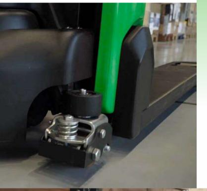
P013i: both the drive wheel and the caster wheels have safe foot protections as standard
